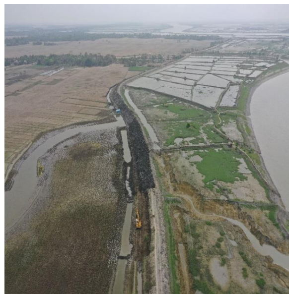
Figure 2-5: Damaged Polder 7/2 (Drone Survey View)
