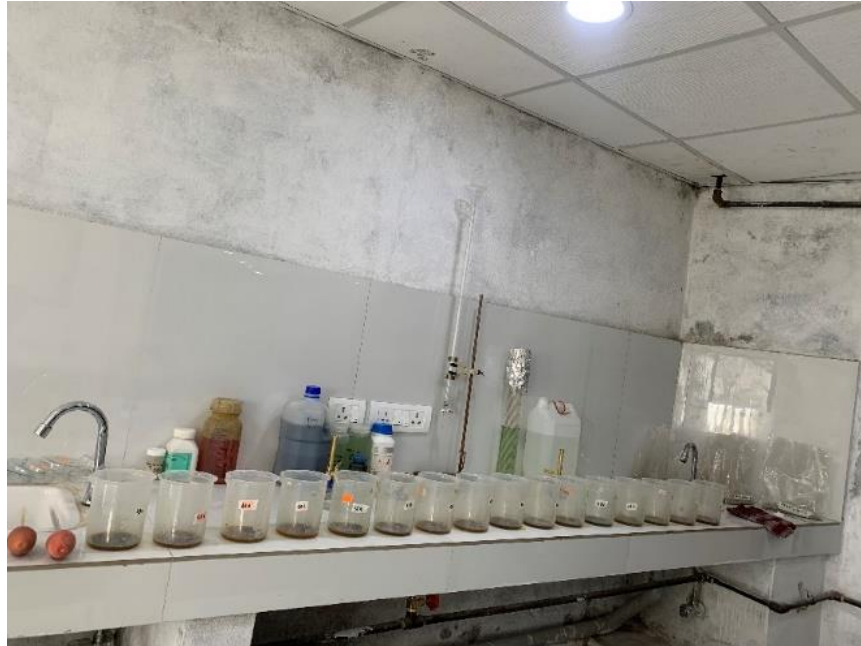
Photo Plate 9: Conducting experiment to calculate Organic matter content in soil
