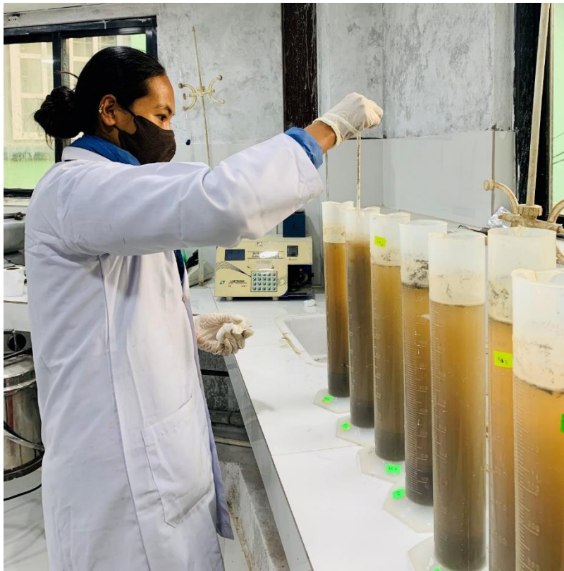
Photo Plate 16: Taking reading for Texture by using Soil Hydrometer
