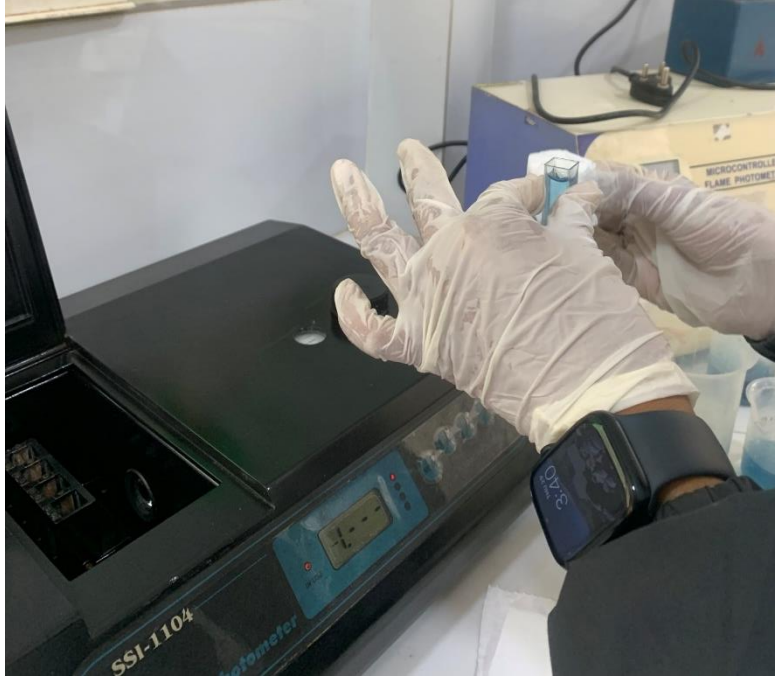
Photo Plate 15: Taking reading of phosphorus in Spectrophotometer
