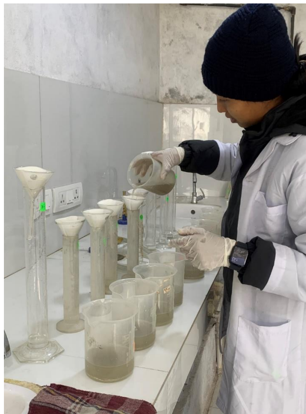
Photo Plate 12: Filtering samples for K analysis
