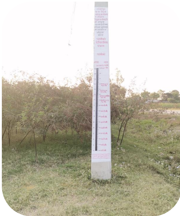
Pole showing historical water level data
