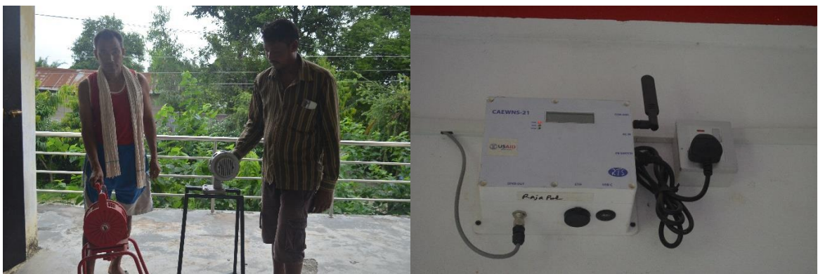
Manual siren in ward no.1, Tihuni & Automatic siren in LEOC for Budi kulo
